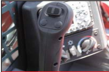
Pilot Operated Controls
