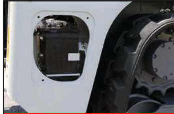
Battery Access Panel
